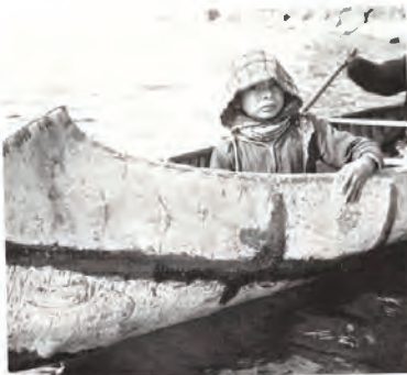
Fig. 2. Boy in a birchbark canoe built by his grandmother, Maria Mikenak, at a time when most of the Northern Ojibwa had been using canvas canoes for several decades. The dark caulking is spruce gum mixed with lard and charcoal. Photograph by John Macfie, near Osnaburgh House on the Albany River, Ont., 1956.
